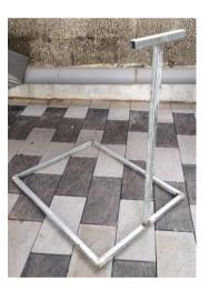
The frame is constructed using mild steel hollow square pipes welded together. All the mountings on the machines are fitted to a steel frame. Holes required to fit other parts of the machine are drilled according to the design.
