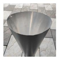
The hopper is made up of mild steel material. The such a way that the feed will fall on to the auger below by gravity. The hopper is of trapezoidal
